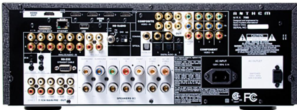
Elsewhere there are five digital audio inputs (three optical, two coaxial) and two outputs (one of each type), six sets of analogue stereo inputs and two outputs, 7.1-channel pre-outs and zone 2 output. On the video side you get three sets of component video inputs and one output, plus three composite video inputs and three outputs. A 12V trigger, RS-232 and IR sockets have custom installation covered, while a radio antenna jack and an input for an optional iPod dock complete the line-up.
