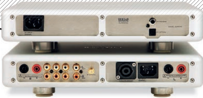
ABOVE: The rear panel for the CD transport has just coaxial and optical digital outputs, while the amplifier sports a Bluetooth wireless antenna as well as three line input phono pairs, an outboard PSU socket and wide-spaced 4mm speaker terminals
